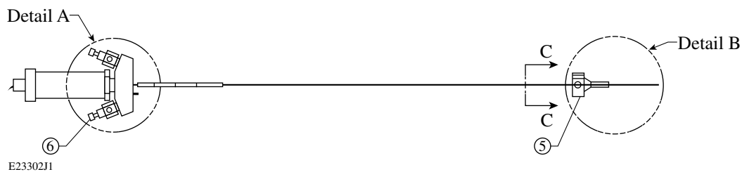
Figure 4.6 Gas-filled target configuration from LLE drawing D-EA-G-354 showing critical dimension of fill hose.
