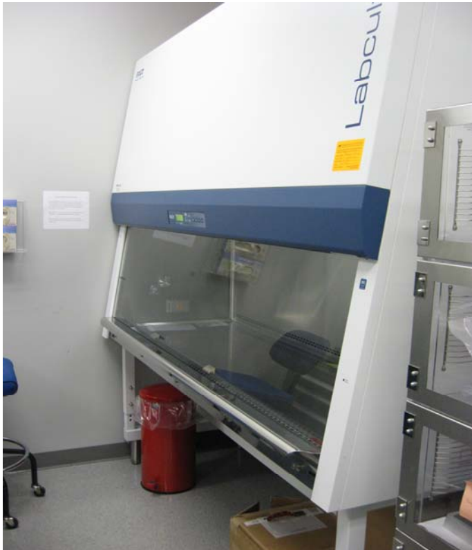
Fig. 1: Exterior view of ESCO Labculture biosafety cabinet used as a BWS in the OMEGA EP Diagnostics Workshop (Rm 6106).
