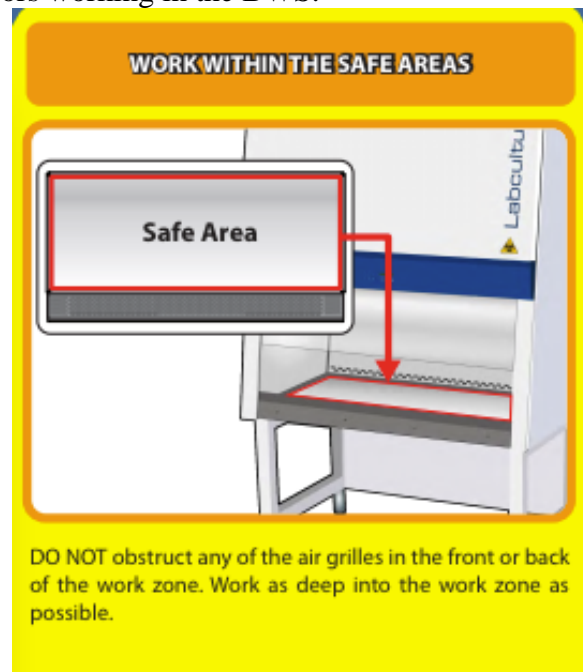
Fig. 4: Airflow patterns in the ESCO BWS. Work should be conducted only in the safe working area (outlined in red). The air grilles (indicated in green) must not be blocked with materials or equipment in order to insure proper airflow in the workstation and minimize turbulence.
