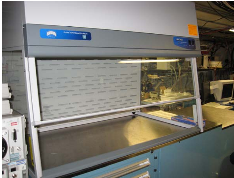
Fig. 5: LABCONCO Purifier® Biosafety Cabinet deployed in LaCave.
