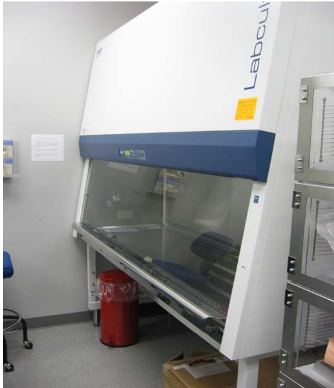
Fig. 1: ESCO Labculture biosafety cabinet Model LA26A2 located in the OMEGA EP Diagnostic Workshop (Rm 6106).
