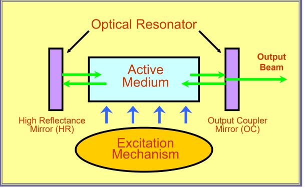
Active medium: This can be a solid (crystal), semiconductor (diode), liquid (dye), or gas, which contains atoms that can emit light by stimulated emission. Also known as lasing or gain medium
