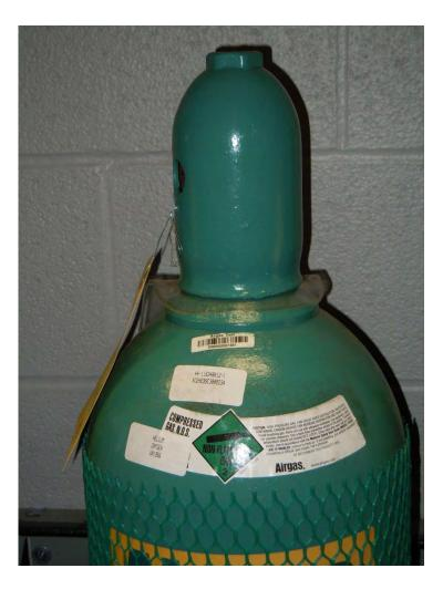
• This is an example of a properly installed cylinder cap
