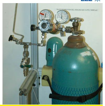
Vacuum fittings are not to be used on pressurized gas systems unless they are specifically rated for pressure applications
