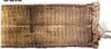
Cut & Tensile Damage
