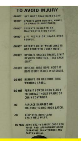
Overhead hoists are to be used in accordance with manufacturers recommendations
